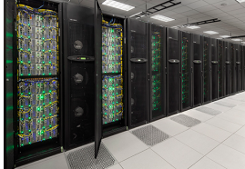
Stampede, U.S.A., #20 with \approx 5 Pflops 56 Gbit/s FDR InfiniBand Fat tree topology 6,400 \times (8 \text{ cores} + 1 \text{ Xeon Phi})
